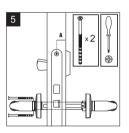
NOTE: This product fits doors thicknesses of 35-80mm. With a 'A' measurement of at least 21mm (see illustration 5). For smaller 'A' measurement 14-20mm use a Code-It spacer (sold separately see part number 59040002).
