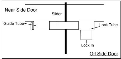
2. With the lock engaged in the slider, mark out position of lock tube and guide tube onto rear door with a pencil, unlock slider, then mark out each hole position. (Use a packer plate as a template to mark hole centres).
