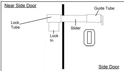
2. With the lock engaged in the slider, mark out position of lock tube and guide tube onto door pillar and side door with a pencil, unlock slider, then mark out each hole position. (Use a packer plate as a template to mark hole centres).
